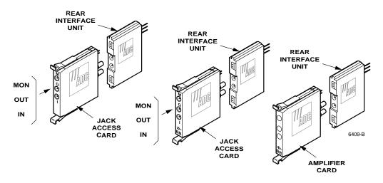
Figure 10. Passive and Active Jack Access Cards
